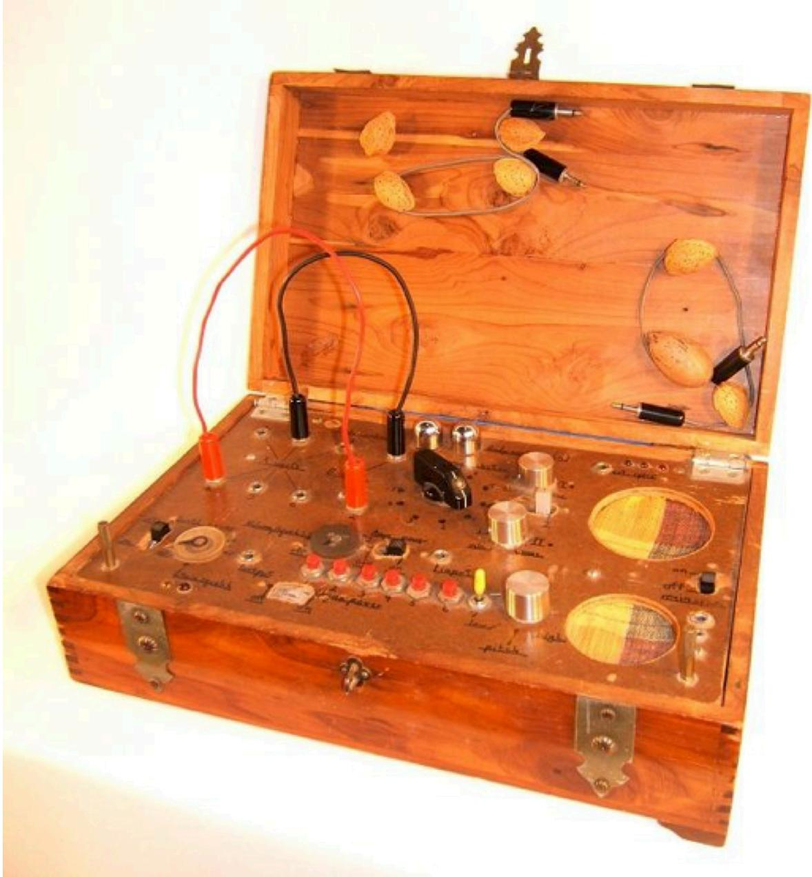
**Illustration 1:** Original circuit-bent amplifier.
